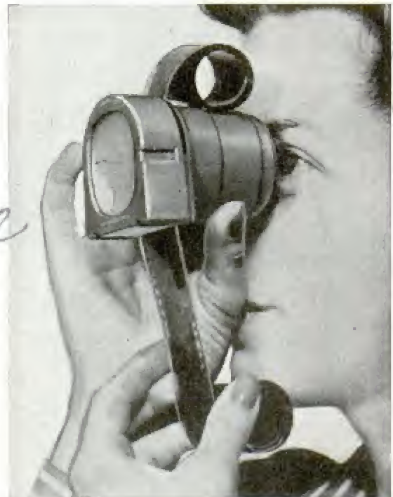
Viewing film while drawing it slowly past eyepiece
